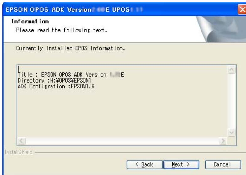
This dialog box displays information on the settings of the already installed EPSON OPOS ADK. Confirm the contents of the list and select the [Next] button if the contents are satisfactory.
